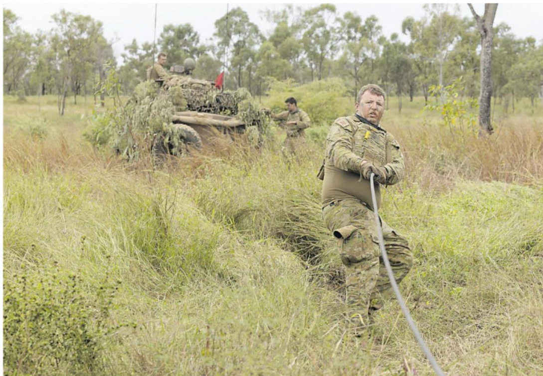
Recovery technician Cpl Alex Cronin, of 2 Cav Regt, carries a winch cable towards a bogged ASLAV during Ex Eagle March at the Townsville Field Training Area. Photos: Sgt Matthew Bickerton
